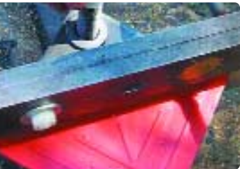
Figure 1: Two 10mm-wide, flat, sharp-edged strips provide the arris armoring with the diamond dowel providing the load transfer for ground-bearing slabs.
